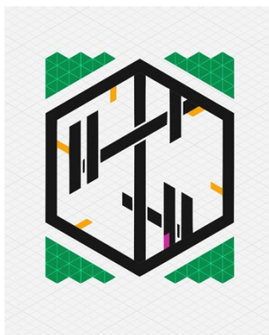
Figure 7. Example of marker developed for the INWIT sites, based on the Vuforia VuMark service. The left part of the image highlights components such as the variable pattern for code registration (green) and the relevant portions used to establish orientation (purple and yellow). Graphics inside the hexagonal border are not used for recognition purposes.
