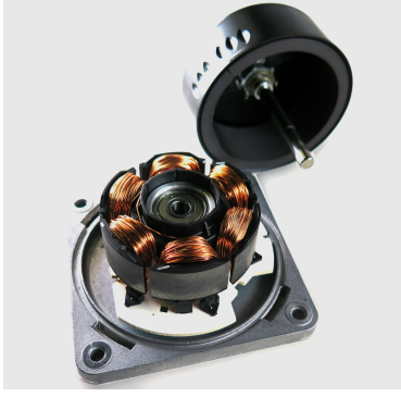
Fig. 1: Motor under test with disassembled outer rotor.
