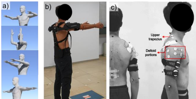
Fig. 2. (a) shows the four static postures considered in the study. (b) shows one subject wearing the MATE exoskeleton in posture P3. (c) shows the positioning of EMG electrodes.
