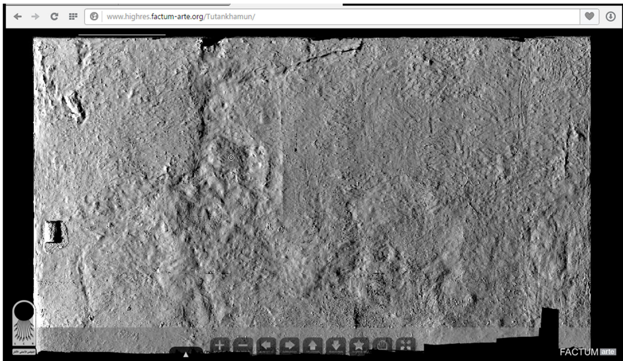
Figure 6: The image of Figure 5 filtered by means of the Retinex tool of GIMP (High Level, Scale 240/6, Dynamic 1,3).
