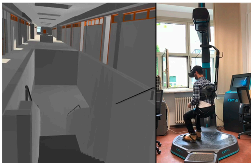
Figure 13. KAT VR platform: virtual reality scenario (left), player setup (right).
