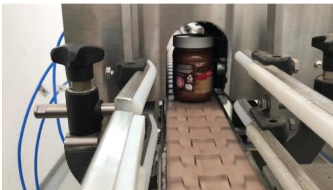
Fig. 2. A chocolate cream jar running below the antennas array, protected by the shielding box
