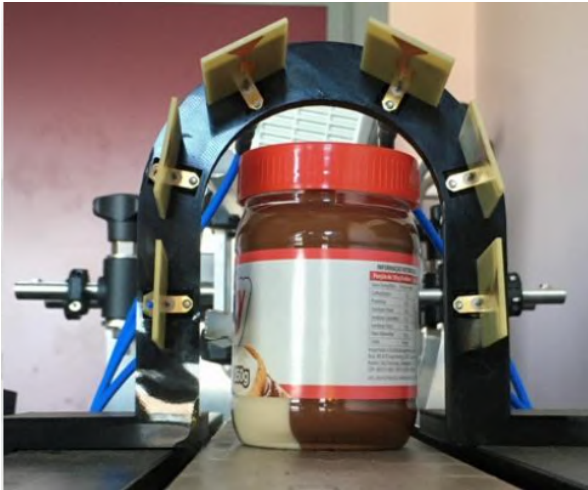
Fig. 1. Antennas array surrounding the item to inspect
