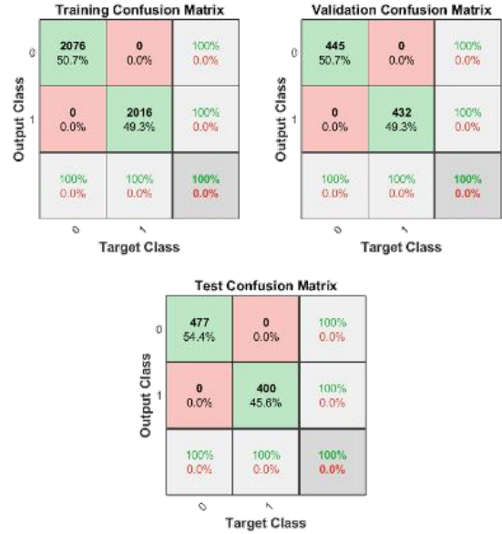
Fig. 6. Confusion matrices obtained by employing all acquired frequencies; the 70% of the total amount of measurements is used to train the neural network, the 15% to validate and a further 15% to test; architecture composed by 2 hidden layers.
