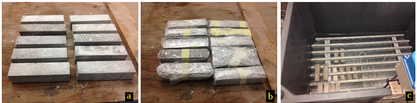
Fig. 5. Curing conditions of some of the tested beams in air at environmental temperature (a), wrapped in cellophane sheet at environmental temperature (b), and in water at controlled temperature (c).
