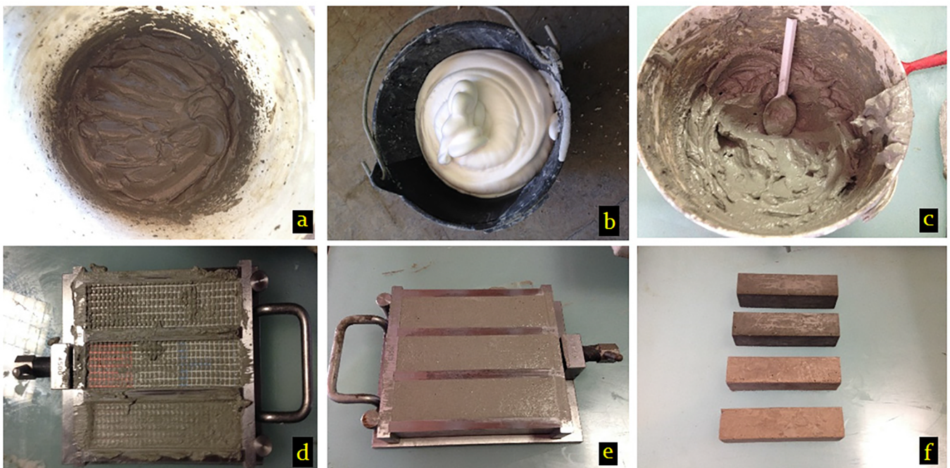
Fig. 4. Photographs of the specimen preparation of foamed concrete beams: a) mix of water, cement and VEA; b) preformed foam; c) paste obtained with a) + b); d) application of bi-directional reinforcement grids; e) covering of the reinforcement grid and completion; f) de-moulding of the specimens.
