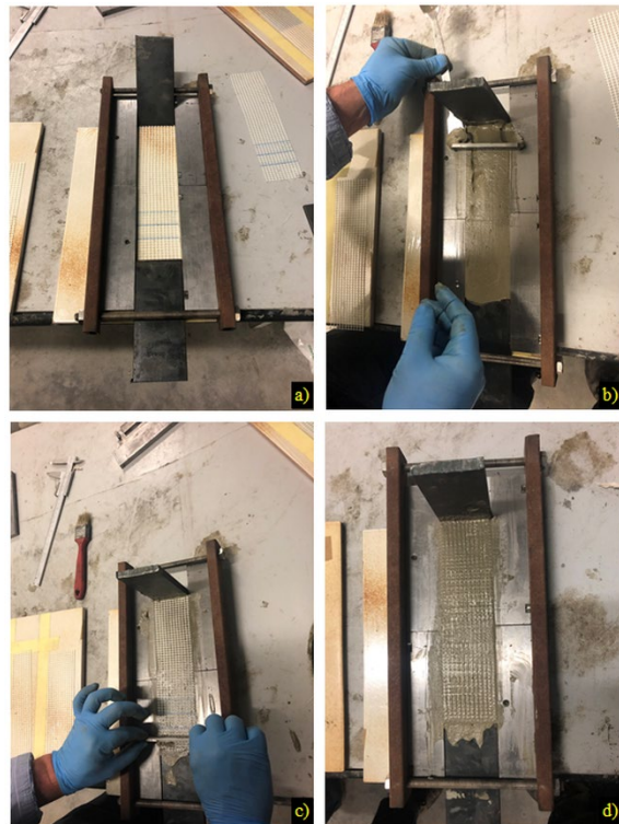
Figure 1. Preparation of samples of FRIL-panels: a) realization of guides and placement of the bottom bi-directional grid reinforcement; b) pouring of fresh E-LWFC paste; c) polishing of the upper surface and placement of the top bi-directional grid reinforcement; d) final samples before removal of guides.
