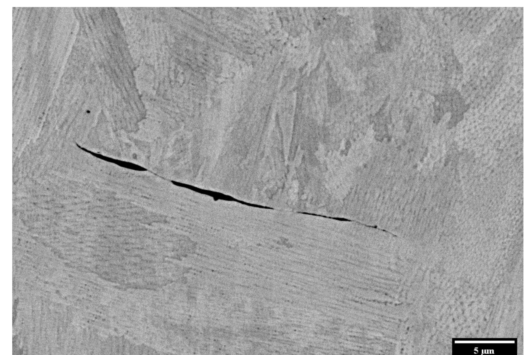
Figure 7. SEM microstructure of a thermal crack grown on a grain boundary.
