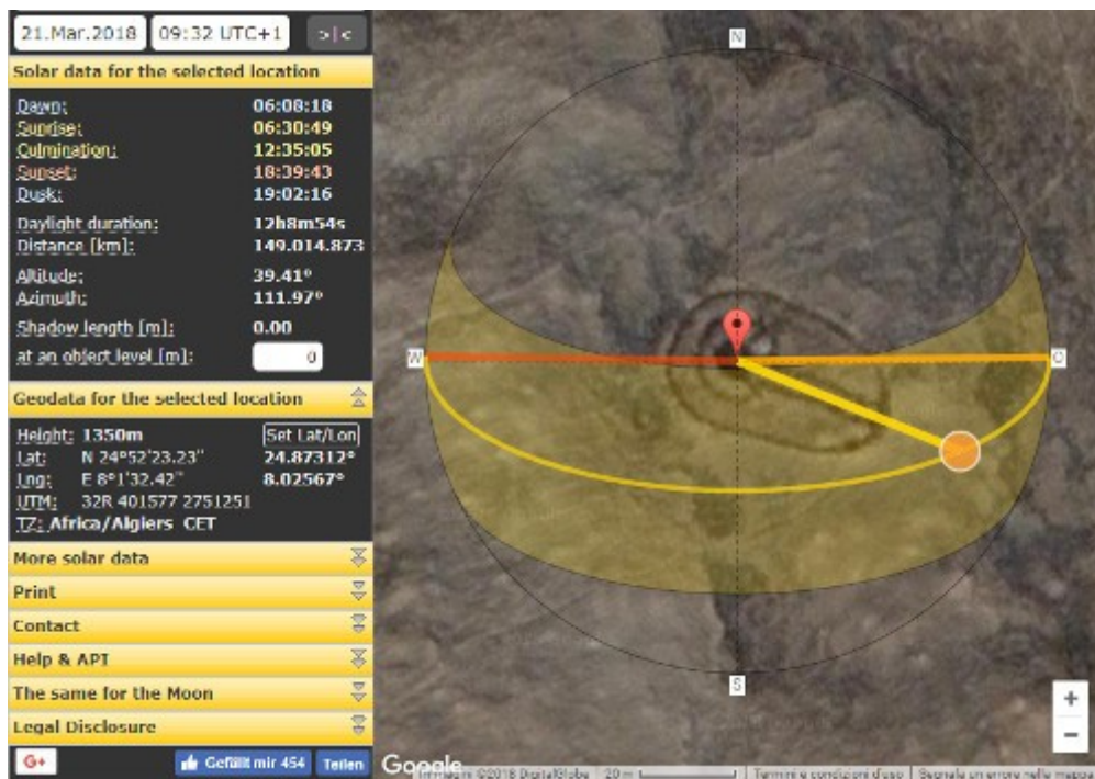
Figure 5: We can use software suncalc.org as a “pair of compasses”. We can read directly the azimuth of the pathway. To measure, it is enough to align the solar azimuth along it, moving the cursor that we can find in the web page. In the case of the figure, the software panel gives an azimuth of 111.97 degrees. Using suncalc.org, it is not necessary to save the Google Earth image and use GIMP.
