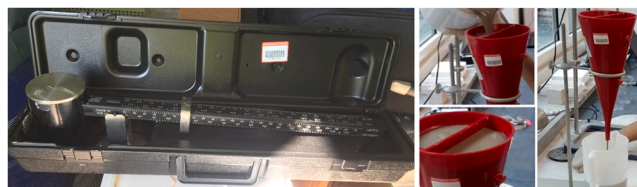
Fig. 3. Mud balance (on the left) and the Marsh cone (on the right). Pictures modified from [30].
