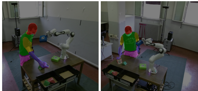
Fig. 1. Example of human-robot collaboration scenario acquired with a multi-view camera setup. Overlaid on each image, the segmentation output of our multi-view human parsing system.
