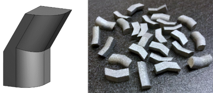
Figure 4. AlSi10Mg sample parts produced via LPBF process for the automotive sector.
