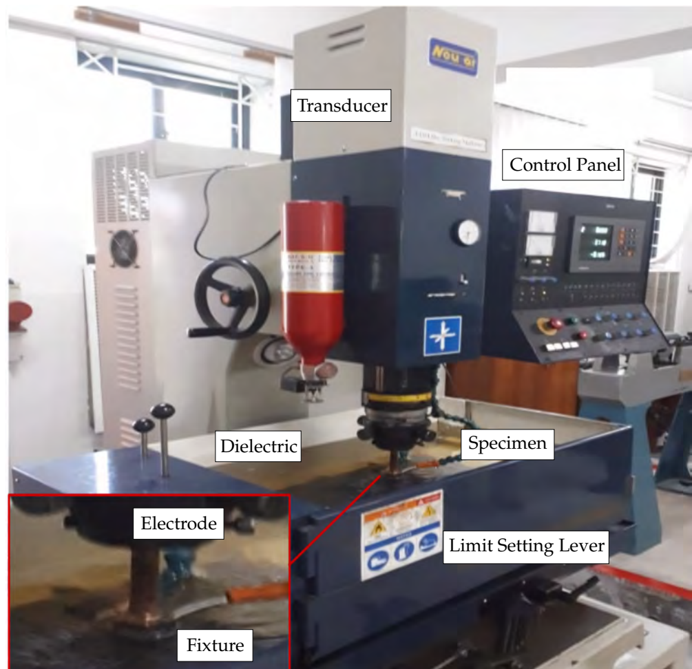
Figure 2. Experimental setup for EDM.
