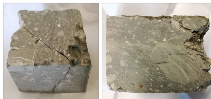
Figure 4. Mélange samples damaged during the cutting phase.
