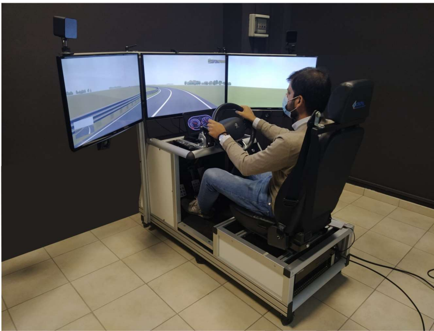
Figure 4. Fixed-base driving simulator of the experiment (Road Safety and Driving Simulation Laboratory, Politecnico di Torino).
