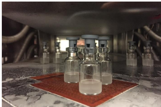
Figure 2. View of the edge sensor on the second shelf of the freeze-dryer.
