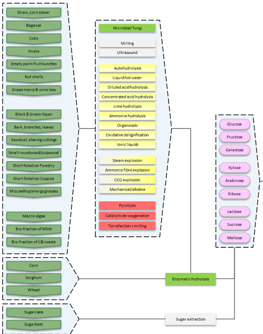
Figure 4: Mapping of feedstock and pre-treatment options to sugars
