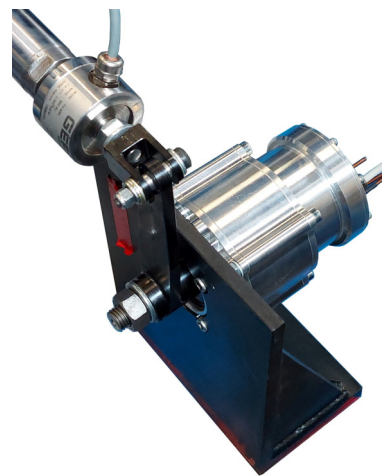
Figure 7. Picture of the rotary electromechanical damper prototype with its linkage.
