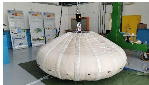
Fig. 18. HIAD demonstrator after inflation testing.
