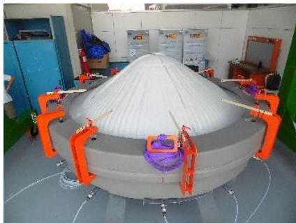
Fig. 19. HIAD demonstrator under static load testing.
