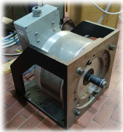
Fig. 6. Automotive inductor motor used for the tests.
