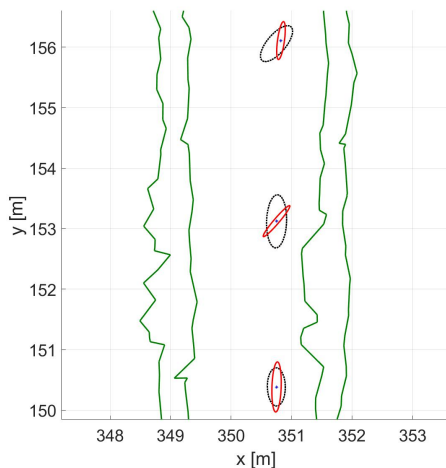
Fig. 8. Evolution of the estimation ellipsoid (black dotted line) and the minimum volume ellipsoid (red line) when data from sensors are fused with the georeferenced information provided by the simplified map of the vine rows (green linestrings).
