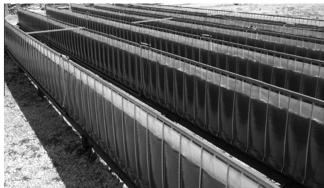
Fig. 2. GWP-II photobioreactor at the F&M facility in Sesto Fiorentino (Italy).
