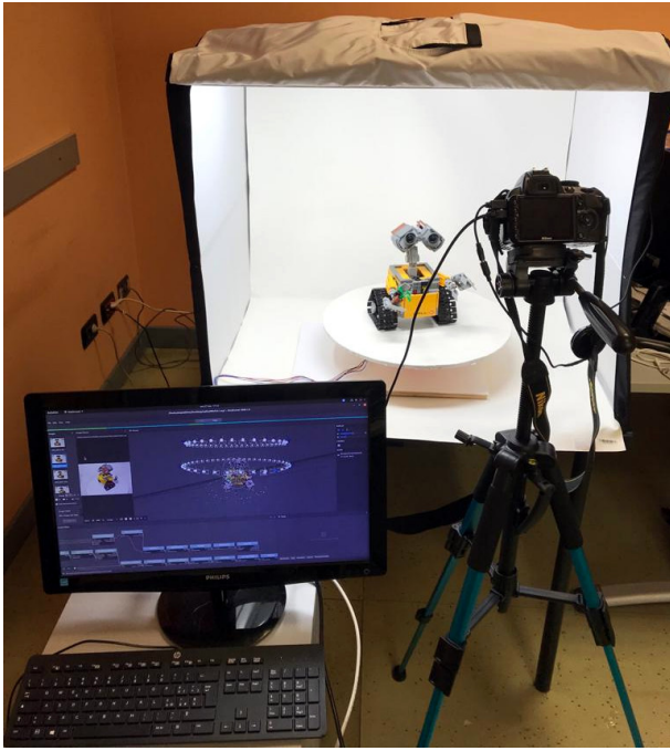
Fig. 1. A typical setup of the proposed acquisition system. The tent front-cover is normally closed during photo acquisition in order to avoid any interference from the environmental light.
