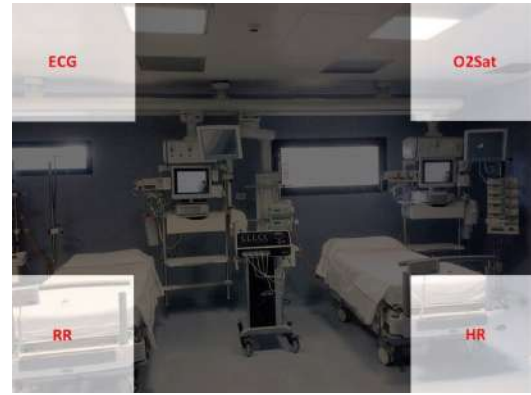
Fig. 9: Flickering squares to select waveforms.
