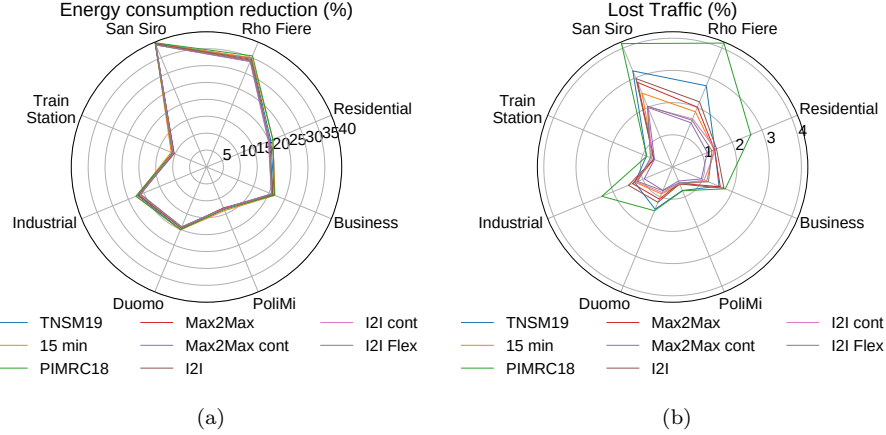
Figure 5: Comparison of dynamic resources allocation strategy in the various areas: (a) Energy consumption reduction and (b) lost traffic.
