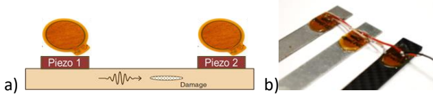
FIGURE 1: a) PIEZOELECTRIC COUPLE WORKING ON A DAMAGED STRUCTURE, b) EXAMPLE OF PIEZO GLUED ON SPECIMENS MADE OF THREE MATERIALS
