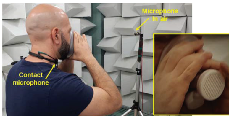
Figure 1 – One of the singer inside the anechoic chamber: the picture refers to the exercises performed with VocalFeel® (a detail of the facemask is shown in the right-side of the picture).
