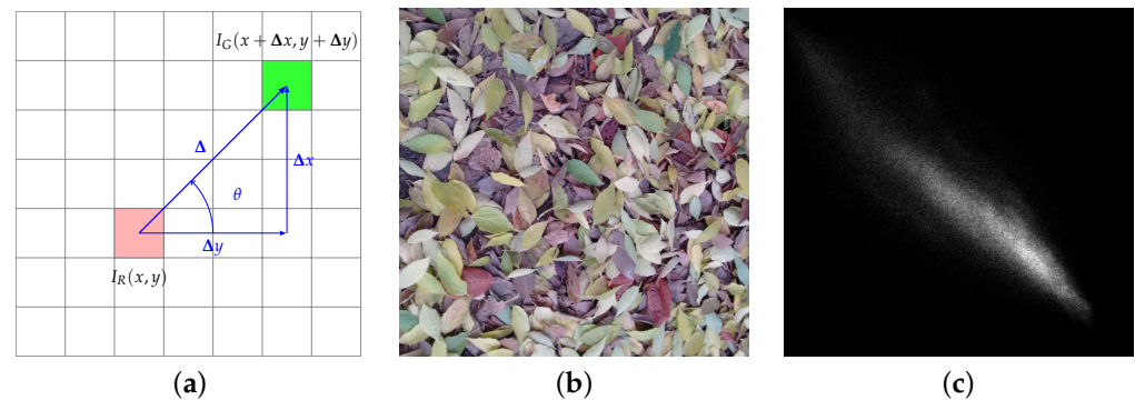
Figure 14. Integrative co-occurrence matrices. From left to right: (a) mathematical formulation, (b) sample image and (c) corresponding inter-class R-G co-occurrence matrix ( \delta = 3\sqrt{2} px, \theta = 45^\circ ). In (a) each square of the grid represents one pixel; (x, y) indicates the coordinates, and I_R(x, y) , I_G(x, y) , respectively, the intensity in the red and green channel. Sample image (b) sourced from the T1K+ dataset [100].
