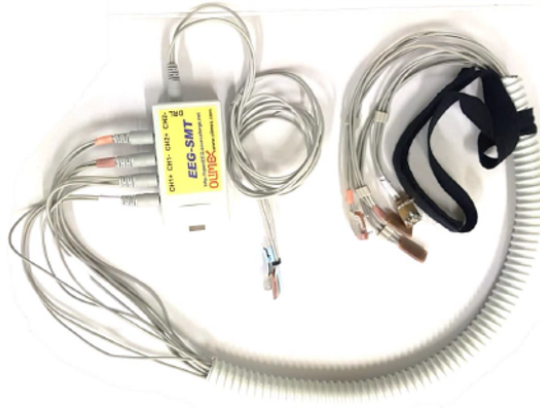
Fig. 2: Low-cost wearable EEG acquisition system.
