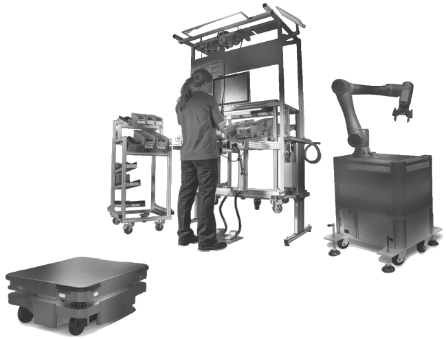
Fig. 1. A robot-assisted assembly use case for the presented collaborative framework. The human operator needs to carry out several tasks performed at ad-hoc workstations. The robotic system observes the operator to determine the current process to infer its own desired behaviour.
