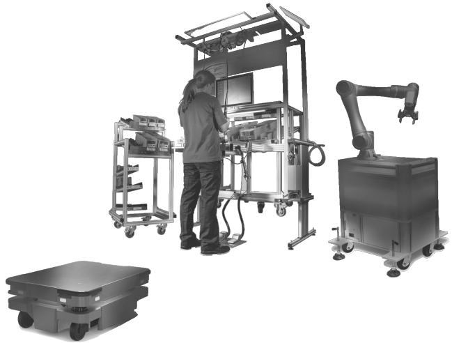
Fig. 1. A robot-assisted assembly use case for the presented collaborative framework. The human operator needs to carry out several tasks performed at ad-hoc workstations. The robotic system observes the operator to determine the current process to infer its own desired behaviour.
