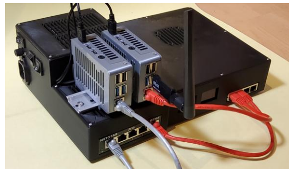
Figure 6: Communications Emulator for the complete subsystem: S-band transmitter, link controller for the iDRS transceiver, Ethernet switch and power supplies, with Ka-band emulated
