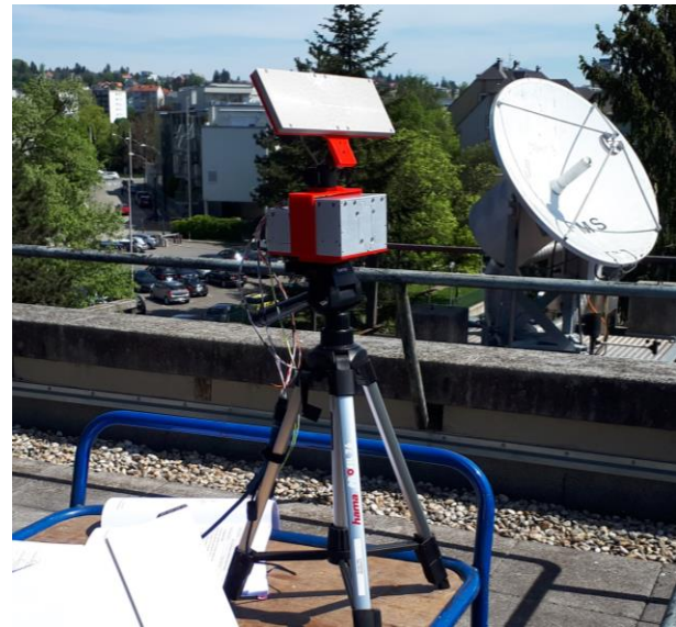
Figure 11: iDRS unit terminal and receiver for the global persistent communications unit hardware in the test-bench
