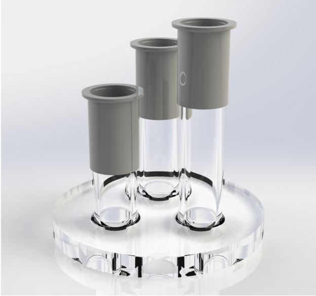
Figure 5: Upper flange with quartz-to-metal connections.
