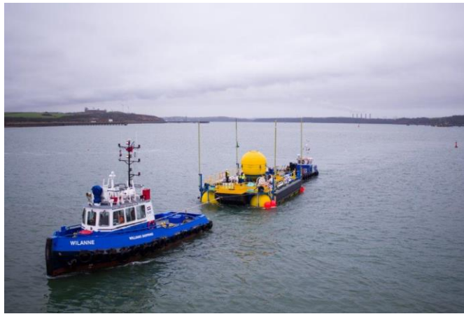
27 28 29 Figure 1: Single float WaveSub on tow, showing the reaction barge in surface configuration with 30 float parked in centre. (Single column image)
