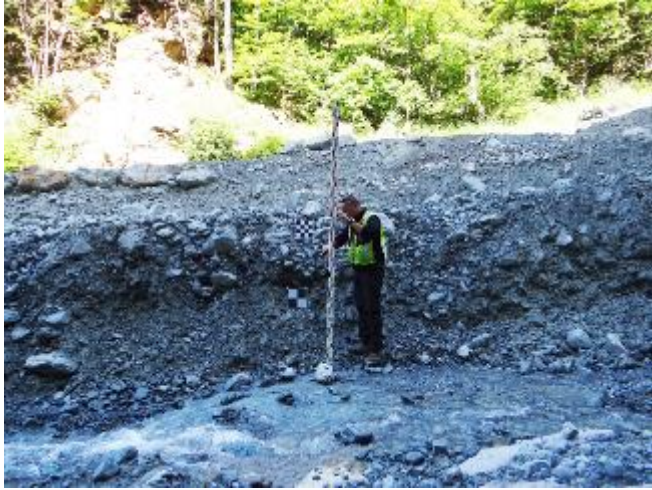
Fig. 5 A portion of the vertical longitudinal trench through the central part of the deposit of the event on 9 June.
