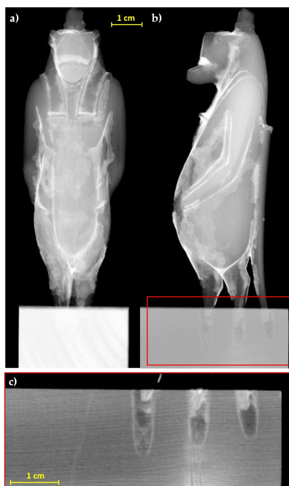
Figure 3. Radiographs of the statuette, (a) frontal and (b) lateral view; (c) detail of the legs and tail insertion in the modern base.
