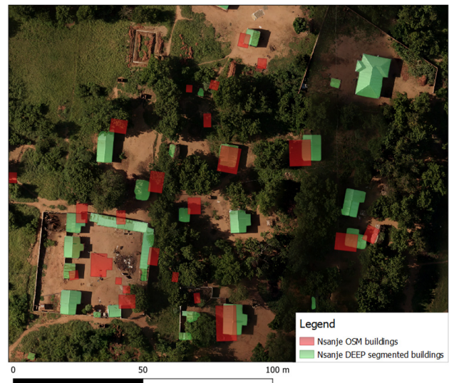
Figure 10. UAV orthophoto of Nsanje (UP4DREAM 2020); superimposed the building footprints generated by AI techniques (in green) and retrieved from OpenStreetMap (in red). It is possible to observe how the OSM data is incomplete and inaccurate compared to the UAV survey's vector data.
