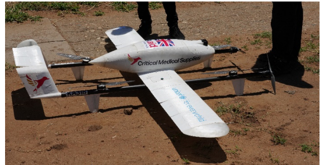
Figure 3. The VTOL UAV used by Swoop Aero in Nsanje.
