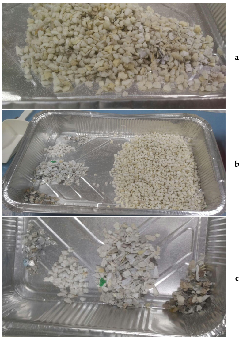
Figure 1. Appearance of the waste polyurethane (PUF) foam: (a) PUF sample collected at the milling unit; (b) PUF sample after the removal of impurities; (c) impurities separated by type.
