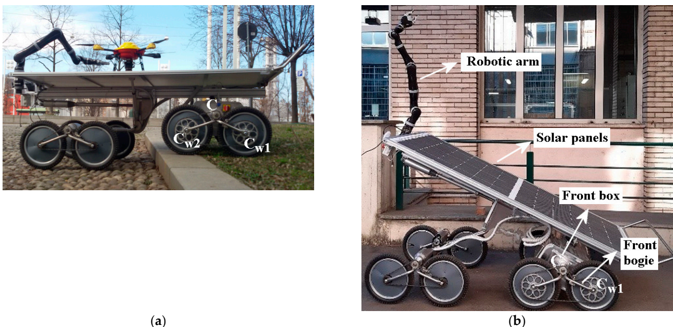
Figure 1. The Agri_q prototype in its standard 8-wheeled configuration: (a) compensation of longitudinal slopes; (b) expansion of the robotic arm workspace.
