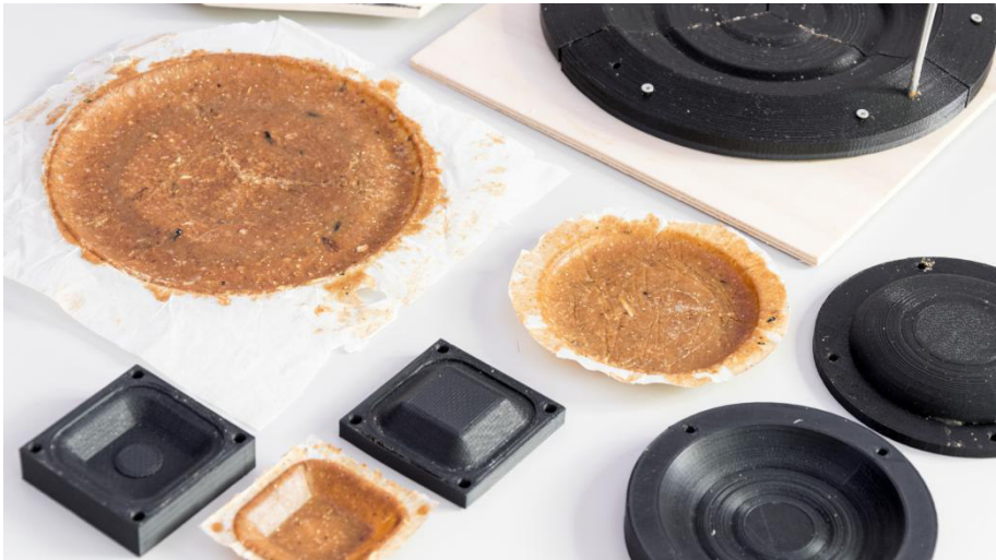
Figure 5. Set of PLA moulds used to give shape to the vegetable polymer.
