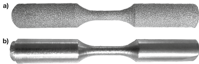
Fig. 5 a An as-built sample and b an AFB treated sample at 6000 rpm for 10 h
