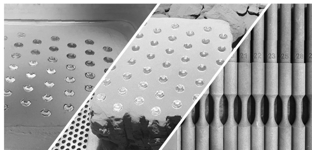
Fig. 2 Samples at the end of the fabrication phase inside the building chamber (last layer), during powder removal in the powder recovery system (PRS) and before finishing
