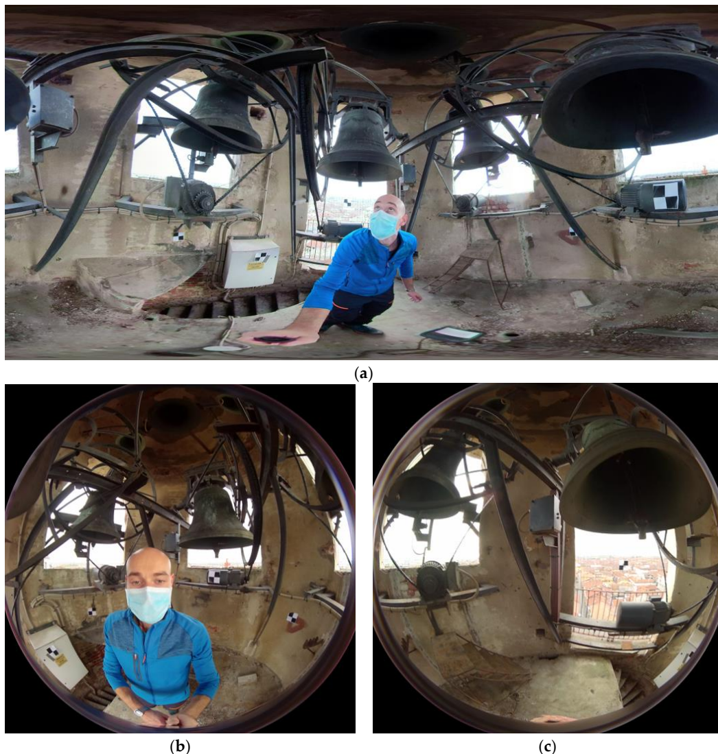
Figure 10. An example of the frames extracted from the 360° acquisitions. A stitched image from the GoPro Fusion (a) and two images extracted from the single camera of the Kandao Qoocam (b,c).
