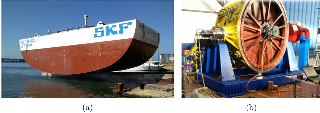
Figure 1.20: ISWEC device installed in Pantelleria island (Sicily, Italy): hull (a) and gyroscope (b).
