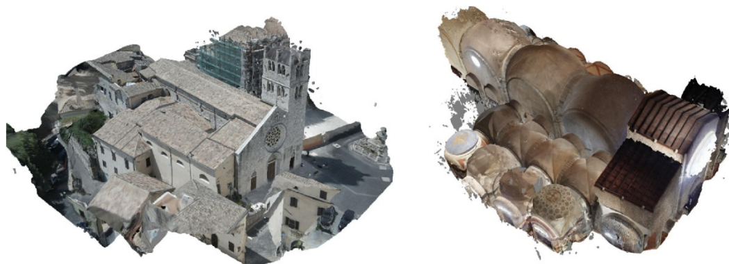
Figure 2. High-density point cloud with applied texture of the: (left) exterior and (right) interior of the church of Santa Maria Maggiore [101].
