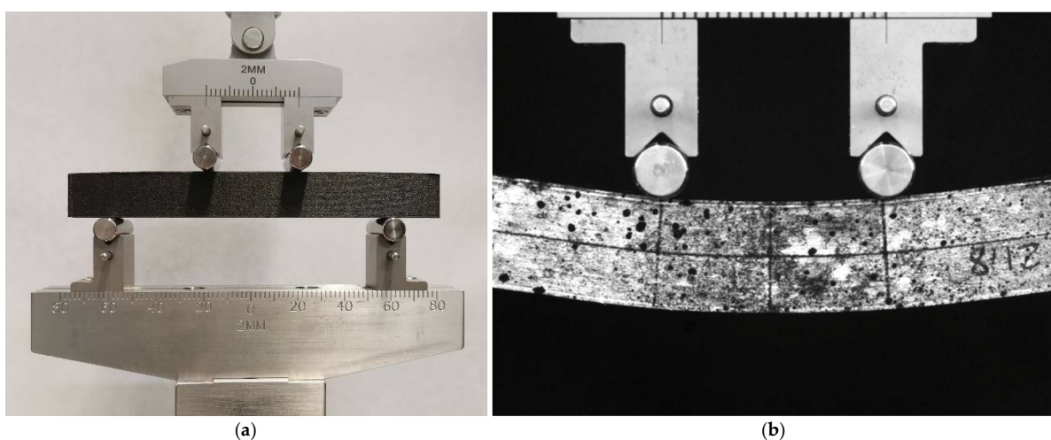
Figure 6. Experimental setup for four-point bending tests on 3D printed structures (a). For each sample, the image sequence of the test was acquired with a 5 MP Pixelink USB camera, and the surface of the sample was painted to allow digital image processing and obtain the displacements (b).
