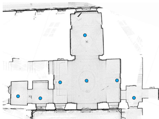
Figure 5. Positioning of the scanning stations inside the atrium of the Capris di Cigliè Palace. To these scans must be added those carried out in the street and in the courtyard. (processing by C. López González).
