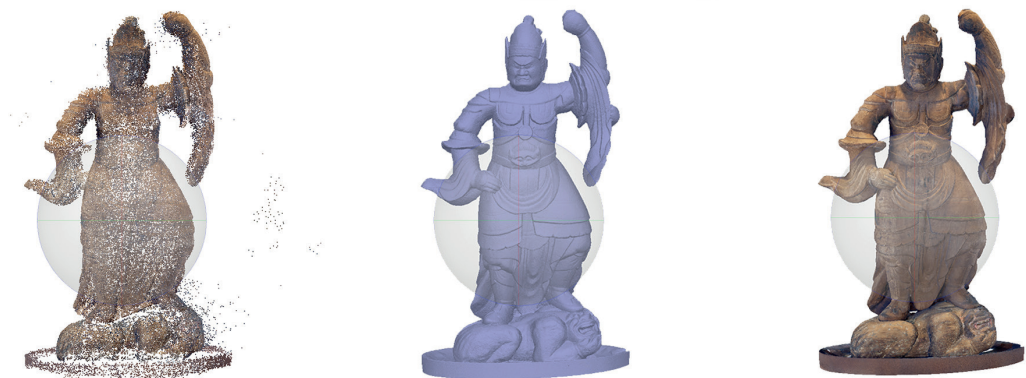
Fig. 5. Creation of dense cloud, mesh model, textured model (digital elaboration by S. Tamantini).
