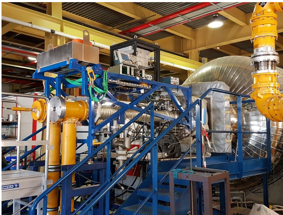
Figure 5. WEST ICRH Antenna Q4 installed in the TITAN vacuum chamber. The high power RF input (visible at the right side in yellow) is not yet connected to one antenna side.
