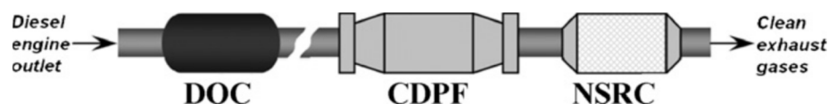
Figure 21. Scheme of the train of monolithic aftertreatment devices. Reprinted with permission from ref. [140]. Copyright 2010 Elsevier.
